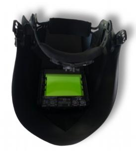
The helmet is equipped with an auto-darkening filter in the highest optical class 1/1/1/1 with protection against IR and UV radiation and stepless adjustment of sensitivity, delay and shade level in the ranges DIN 4-8/9-13.
